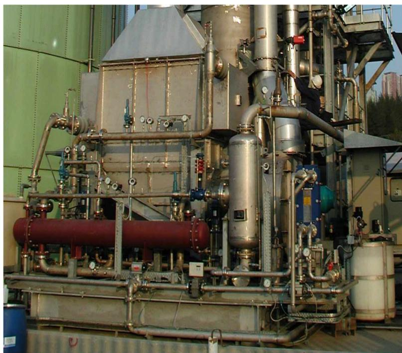
stage to stage in the evaporator unit. The concentrate from the final stage can be drawn off and fed to a drying system or dewatered with a filter-press.
